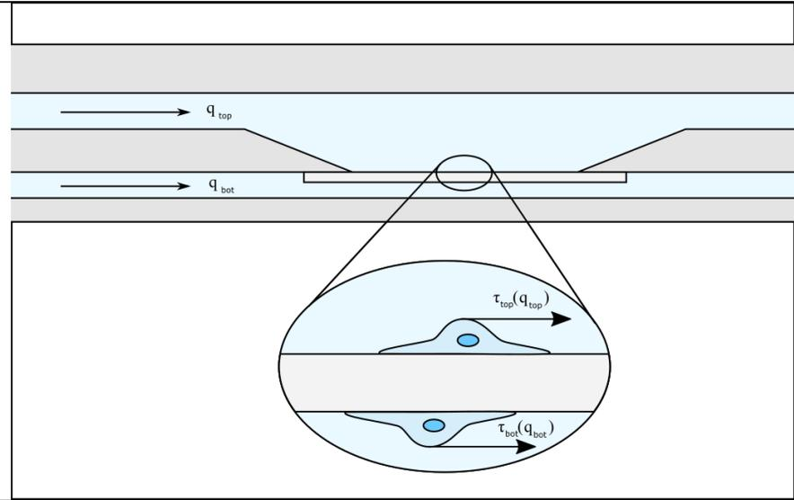
Cells cultured on the membrane are mechanically stimulated by the fluid flow. The different heights of the channels result in varying stress on the cells (for the same flow rates).
