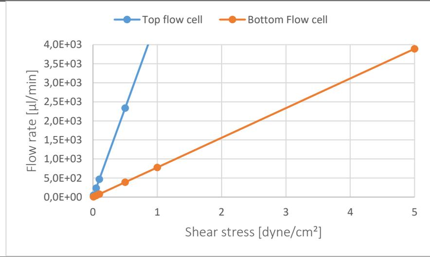
The curves representing the flow rate as a function of shear stress on the membrane in the two channels is reported in this graph.
