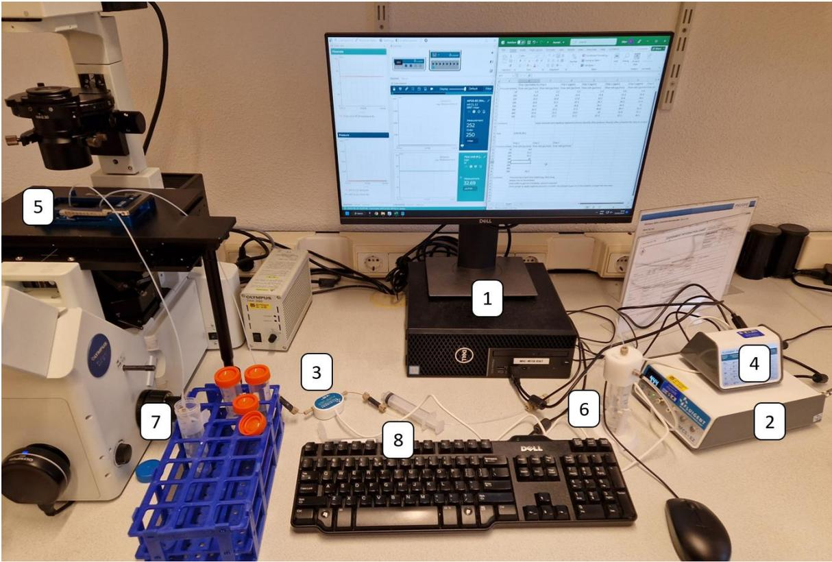
Figure 4: The setup used to determine the permeability of the Micronit EOR chips
