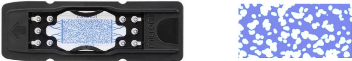
Figure 1: The physical rock EOR chip (left) and a zoom-in of its pore structure (right)
