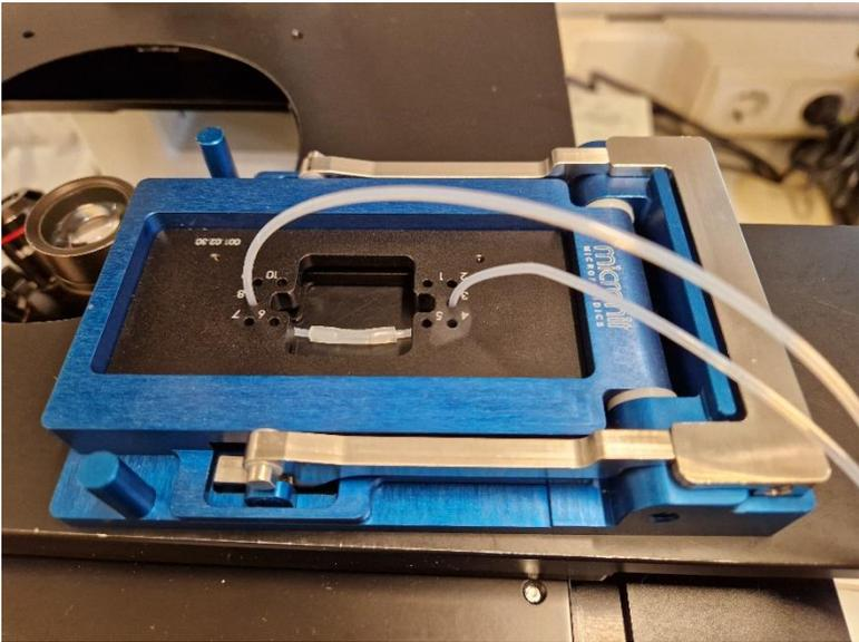
Figure 5: In the zero measurement, the EOR chips has been replaced by a piece of silicon tubing with a negligible resistance
