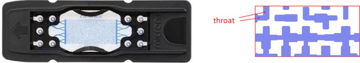
Figure 2: The random network EOR chip (left) and a zoom-in of its pore structure (right)
