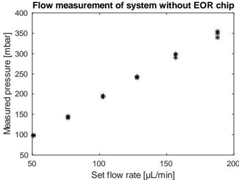
Figure 6: The measured pressure drop over the system without EOR chip plotted against the set flow rate
