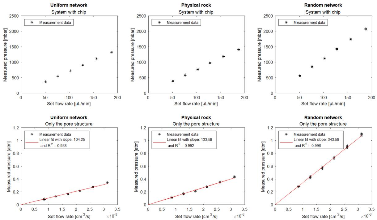
Figure 7: First row of graphs: the measured pressure drop over the system including an EOR chip plotted against the set flow rate. Second row of graphs: the same as the first row of graphs, but now the pressure drop from the system and the estimated pressure drop over the EOR chip its channels are subtracted so that we obtain the pressure drop over the pore structure only
