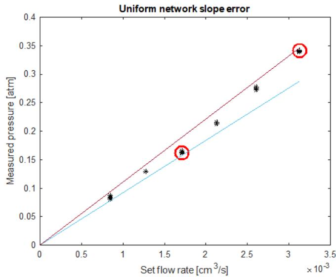
Figure 8: Error determination for the permeability in the uniform network EOR chip
