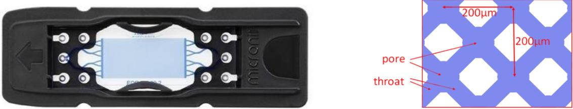
Figure 3: The uniform network EOR chip (left) and a zoom-in of its pore structure (right)
