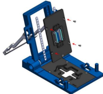
**3)** Place and fix top insert. Use the 0.5mm spacers between the top insert and Fluidic Connect Pro.
