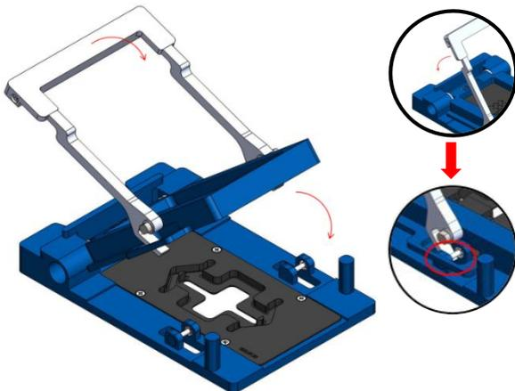
**4)** Close the holder using the handle and fix the assembly using the gripper.
