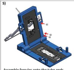
Assemble ferrules onto the tube ends
