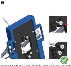
Press the tube with ferrule into the top insert
