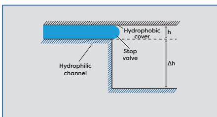
**Capillary stop valve cross-section**
